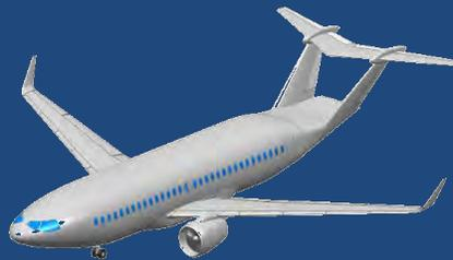
The "**double bubble**" aircraft **design concept** developed by Aurora Flight Sciences, MIT and NASA, and currently being funded through the CLEEN Program, is demonstrating how aircraft configuration changes can provide a **step change in noise and fuel use**
