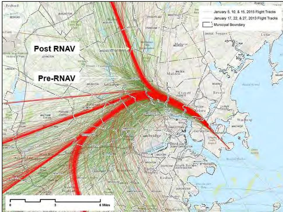
Figure 2.7(b)-2 Flight Tracks, Before and After RNAV
