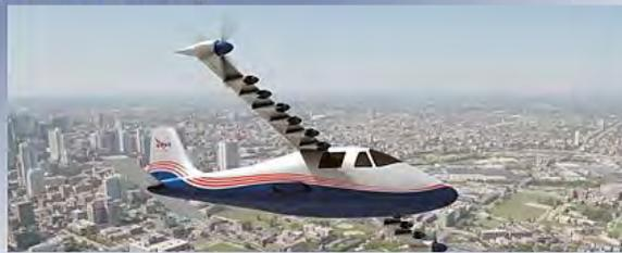
The goal of the X-57 is to demonstrate a 500 percent increase in high-speed cruise efficiency, zero in-flight carbon emissions, and flight that will yield significantly reduced community noise
