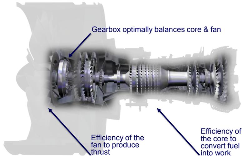
Engine Efficiency  $\approx$  propulsive efficiency x thermal efficiency
