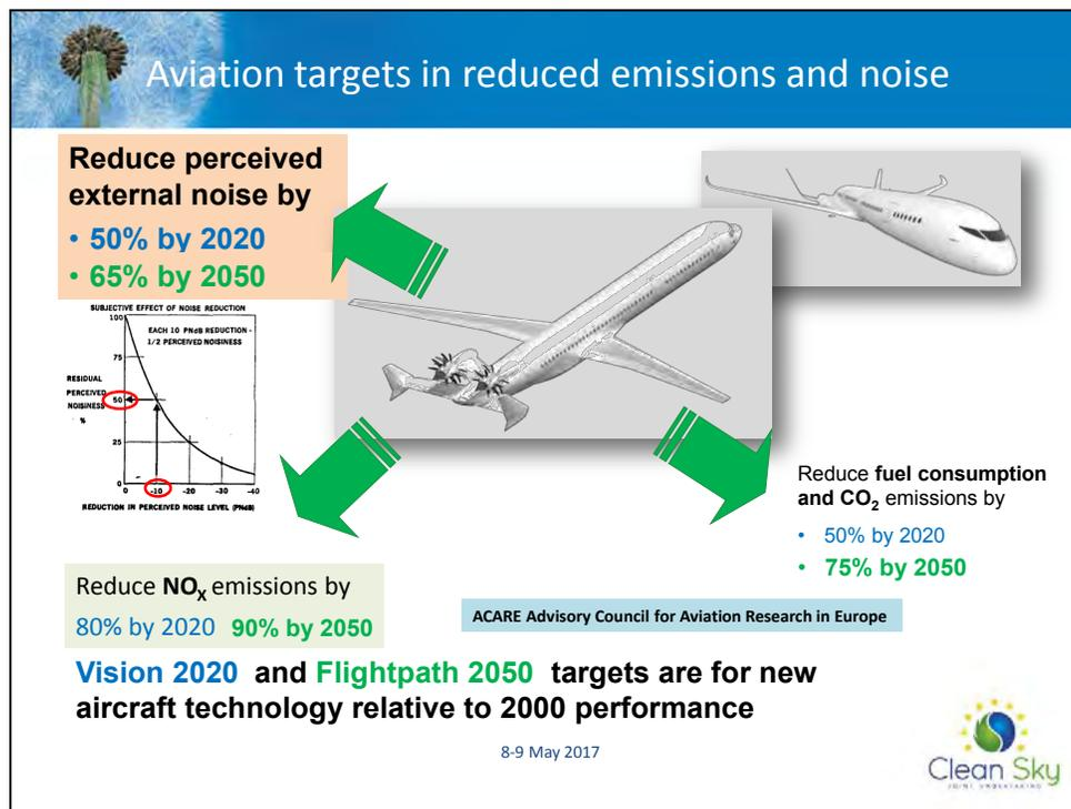
Figure 3.7-1 Aviation Targets: Reducing Noise and Emissions
