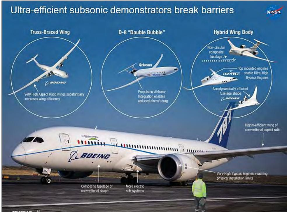
Figure 3.4-8 Ultra-Efficient Subsonic Configuration Options
