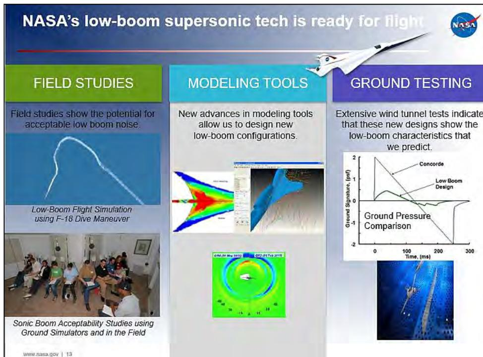
*Figure 3.4-7 Low-Boom Supersonic Technology: Tested and Ready*
