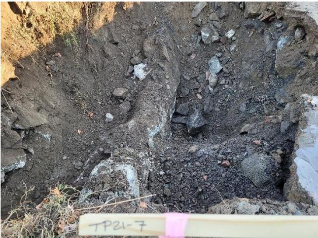
*Photo 17: Image of former concrete foundation element observed in TP21-7, looking west.*
